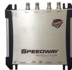
FIGURE 12. Impinj R420 RFID reader.
