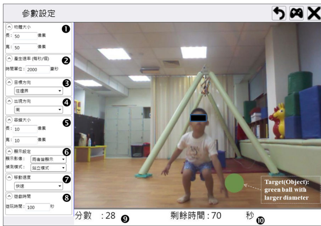
FIGURE 3. Game parameters set of the proposed training system include: ❶ Object Dimension, ❷ Object Occurrence Frequency, ❸ Moving Orientation, ❹ Initial Position, ❺ Tolerance range of Hit, ❻ Skeleton Presentation: Standing or Sitting, ❼ Moving Speed, and ❽ Default Completion Time; moreover, test performance with ❹ Score, and ❺ Remaining Time.
