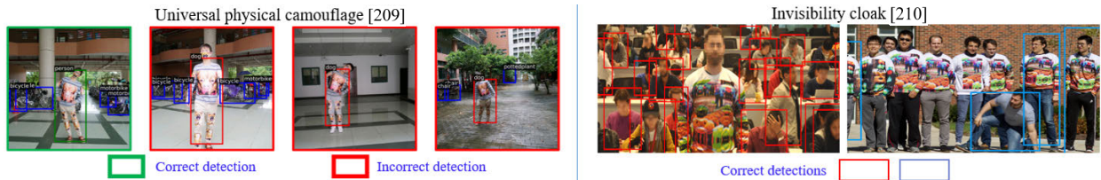
FIGURE 10. Representative attacks on detectors - randomly selected. (Left) Universal adversarial camouflage [209] incorrectly detects the target class at the cost of conspicuous patterns. (Right) Invisibility cloak [210] makes target object invisible with high probability. Images are taken from [209] and [210].
