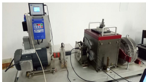
FIGURE 15. Planetary gearbox fault simulation test-bed.
