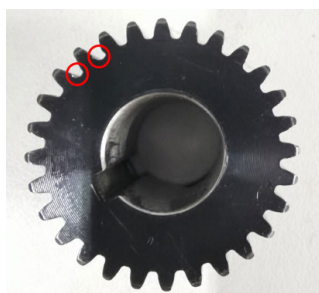
FIGURE 16. Cracked solar wheel.
