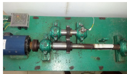
FIGURE 5. Gear fault simulation test bed.
