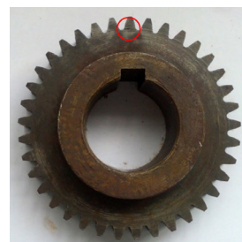
FIGURE 6. The gear with a cracked tooth.
