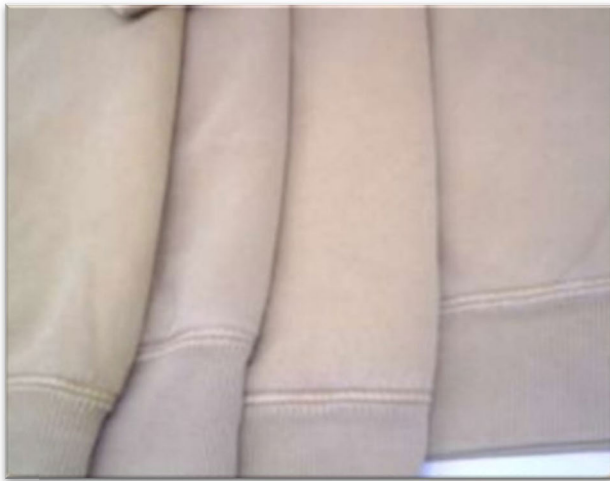
FIGURE 2. Fabric defect: dye-staff absorption.
