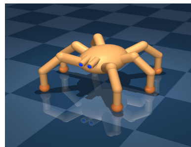
FIGURE 2. Hexapod agent in our study. It has observations as the joint positions and velocities, torso velocities and orientations, and sensor information (IMU, force, torque). Actions are input to the actuator of each joint.
