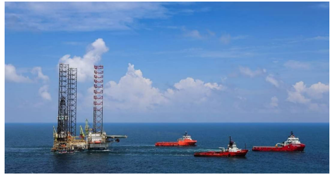
FIGURE 5. Three tugboats brought Tam-Dao 05 to position and maneuvered to correct direction of JuR before anchoring.
