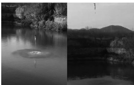
FIGURE 25. TDAV movement exiting the water and hovering.
