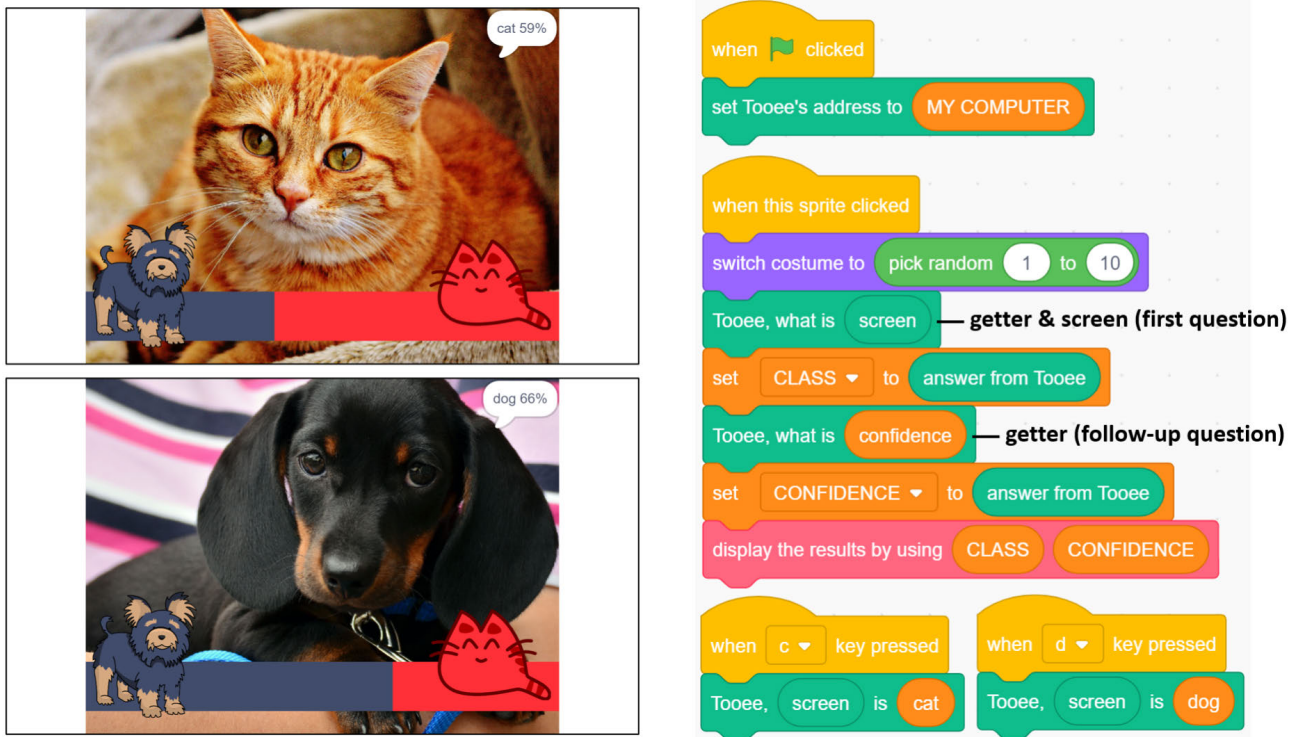
FIGURE 9. Object Classification example for K-12 AI education. When the program starts, a connection between Scratch and Tooee is established. When a user clicks on a background image, the image changes randomly, and the program determines whether this image is a cat or a dog based on the confidence value calculated by Tooee. The user can train Tooee by pressing the “c” or “d” key.
