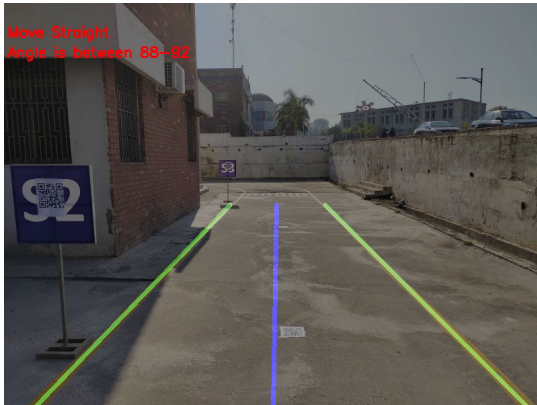
FIGURE 5. Lane Detection using PHT.
