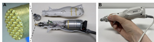
FIGURE 1. (A) Open view of the operator handheld signal probe showing the voice coil motor-controlled and electrode tip and closeup picture of the textured face of the brass signal electrode tip. (B) Use example of the handheld probe.
