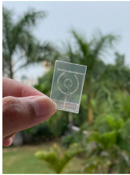
FIGURE 4. Fabricated prototype of single element flexible antenna.
