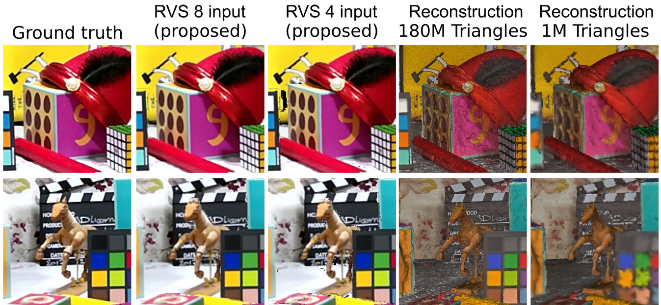
FIGURE 4. Visual comparison between RVS (4 and 8 input views) on zoomed details of Toystable dataset [2] at resolution 1920 \times 1080 and mesh reconstruction (180M triangles, and 1M Triangles, decimated) with associated ground truth. The mesh reconstruction was created with the CapturingReality software [39] using around 500 pictures [40] and is rendered using Phong shading.
