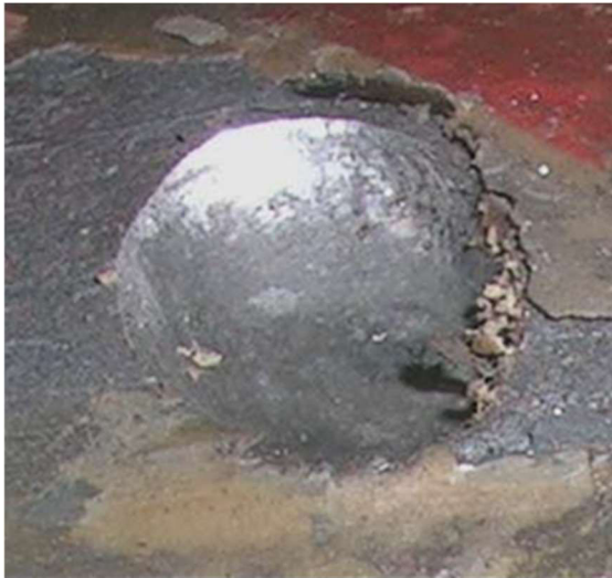
FIGURE 4. An impact crater of 6 mm diameter and 0.83 mm depth on the pipe surface from a 11.5 kg load dropped at 1.5 m height using a spherical indenter.
