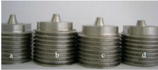
FIGURE 22. Conical-indenters after impact, a) 6.5 kg (0.5 m), b) 6.5 kg (1.0 m), c) 11.5 kg (0.5 m) and d) 11.5 kg (1.0 m).
