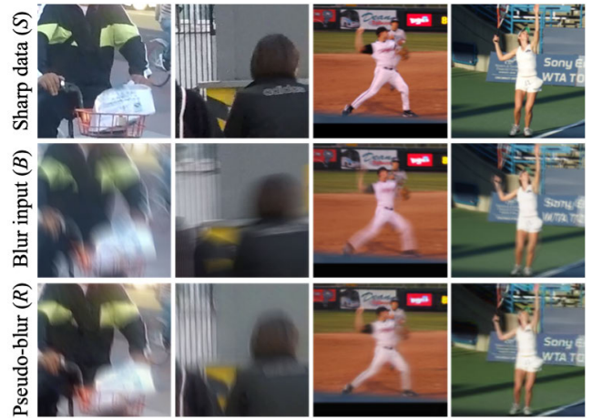
FIGURE 4. Example of our synthesized blurry results ( R ) or pseudo-blurred on the third row using \Omega_T that are different with the blurry input ( B ) in the second row. The first row indicates sharp image input ( S ).
