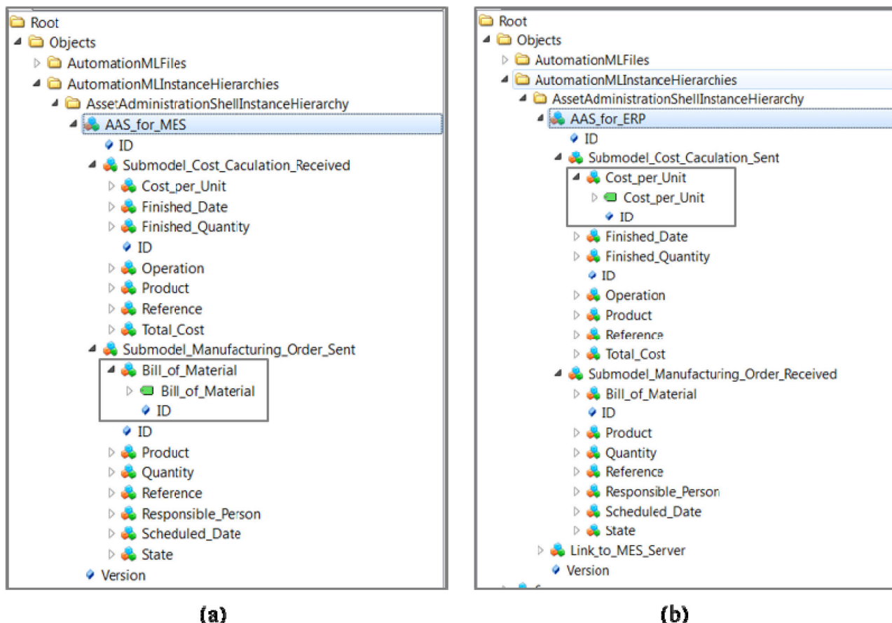
FIGURE 8. AutomationML-based OPC UA information models for the MES and ERP.
