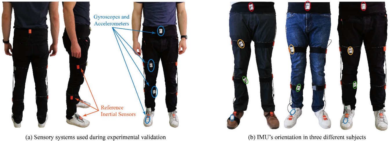
FIGURE 2. Sensor placement during the experimental essays. In panel (a), we highlighted the two sets of sensors involved in the experimental set-up. Orange inertial sensors are the Xsens sensors used as the gold standard for the calculus of the biomechanical model. In contrast, the sensors highlighted in blue are used to acquire the velocity and acceleration from gyroscopes and accelerometers to feed the Kalman algorithm. In panel (b), we show the placement of these sensors in three subjects that participated in the experimental validation. Ellipses of the same color mark the same sensor in each subject. The orientation of the same sensor slightly varied between subjects.
