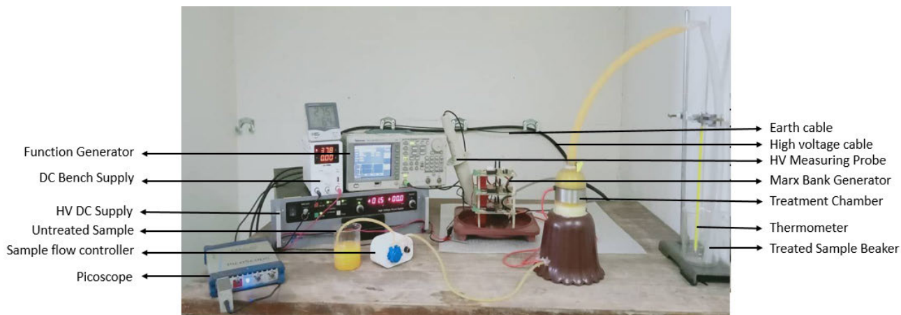
FIGURE 15. Experimental setup of electroporator with continuous liquid flow and double-exponential waveform for orange juice treatment.
