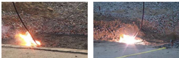
(b) Arc generation during an experiment ((left) dry asphalt, (right) wet sand)
