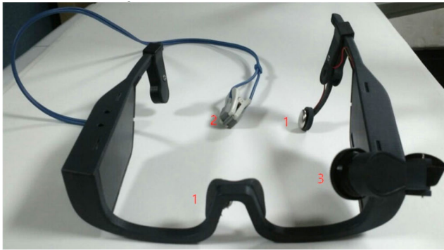
FIGURE 1. Proposed hardware. (1) EDA sensors that measure the skin conductance from the user's nose and mastoid. (2) PPG sensor with an ear clip that measures the pulse of the user's earlobe. (3) Built-in camera that measures the user's facial expressions around the eyes.
