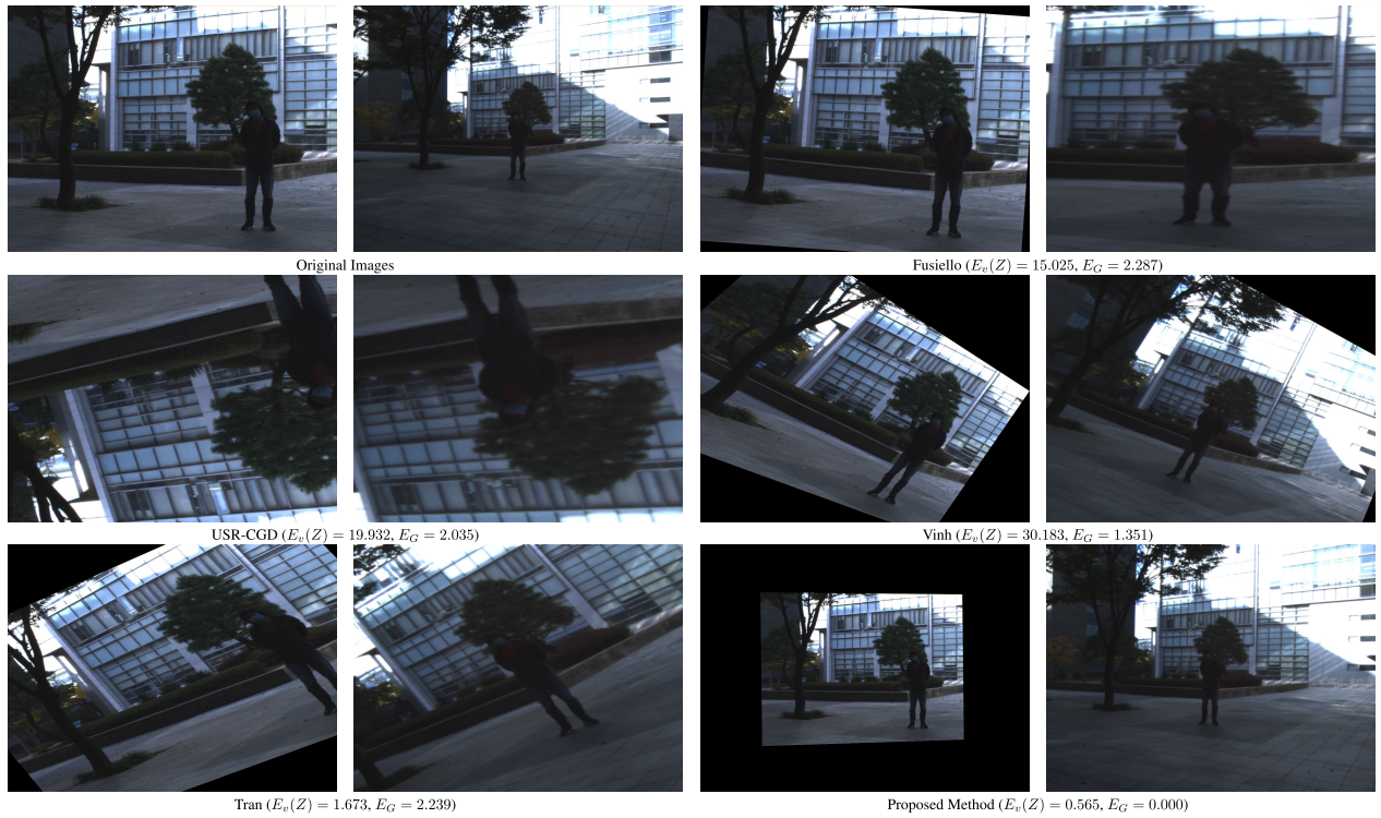
FIGURE 7. Comparison of vertical disparity errors and geometric distortion for 0804_900mm in the SKKU_dFoVs database.
