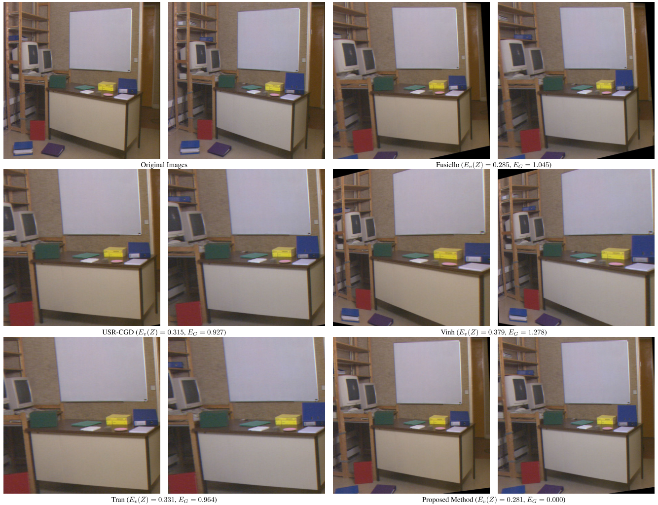
FIGURE 5. Comparison of vertical disparity errors and geometric distortion for Serfaty0_OG2 in the Syntim database.
