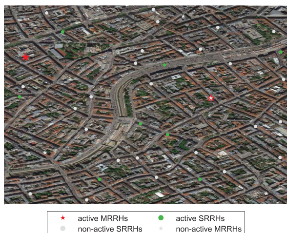
FIGURE 9. Resulting radio network for a C-RAN at 28 GHz with \omega_1 = 0.6 and LT profile.
