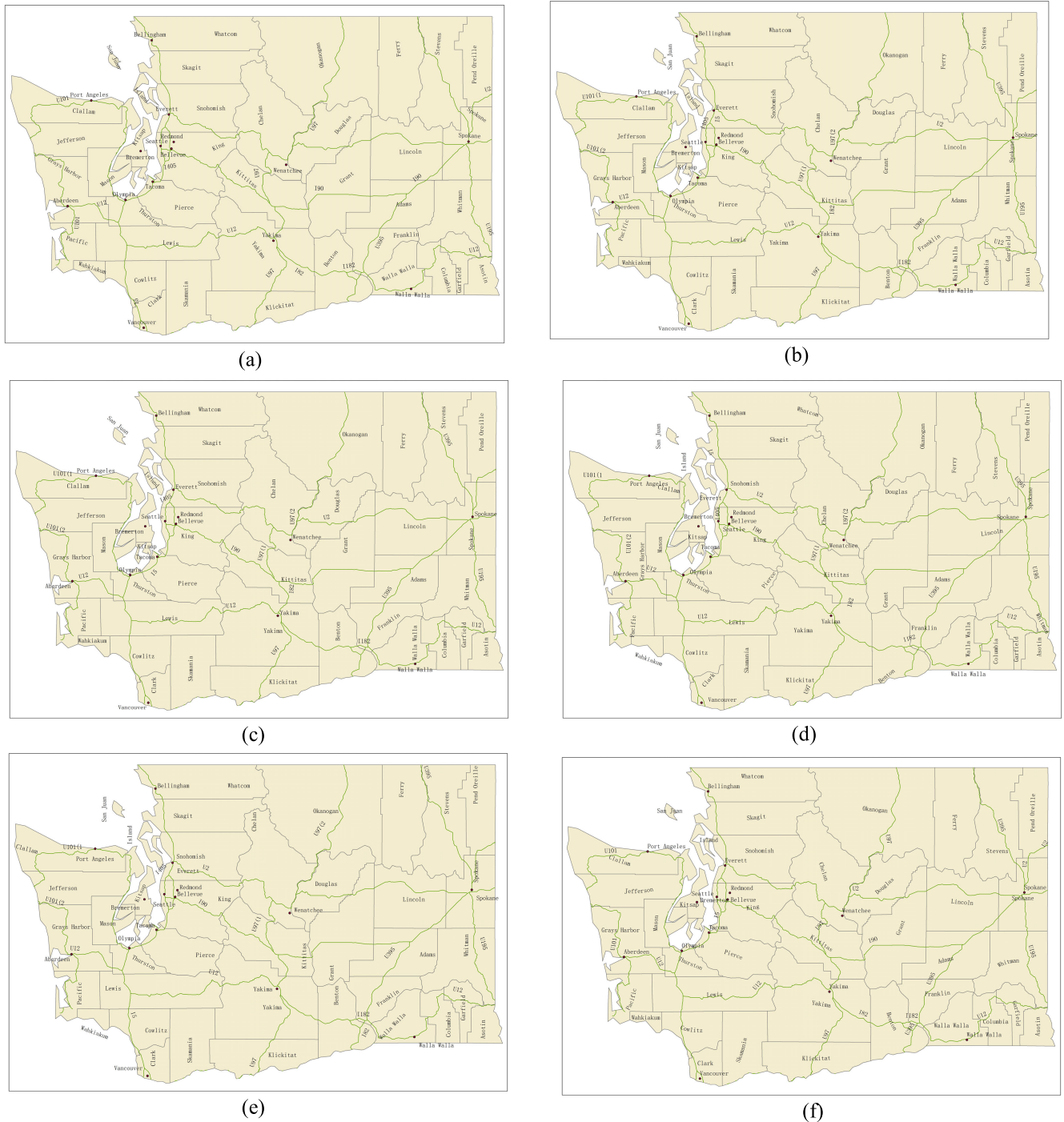
FIGURE 7. The map of Washington State with labels generated: (a) DDEGA-LU [2]; (b) DDEGA-NM-300 iterations ( N = 8, M = 1 ); (c) DDEGA-NM-10000 iterations ( N = 8, M = 1 ); (d) DDEGA-NM-300 iterations ( N = 8, M = 3 ); (e) DDEGA-NM-10000 iterations ( N = 8, M = 3 ); (f) Maplex.
