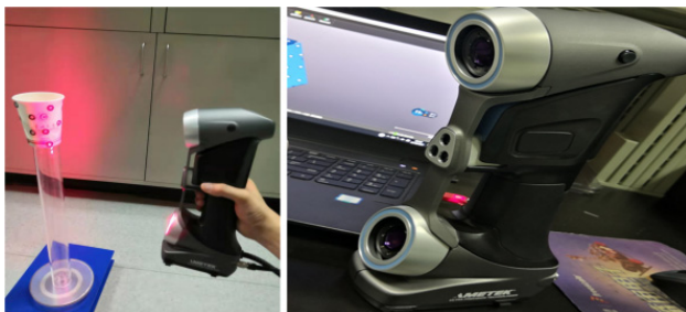
FIGURE 2. Scanning process and HANDYSCAN 700TM portable laser scanner.
