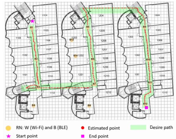
(b) Track 2: Floor detection with barometer readings.
