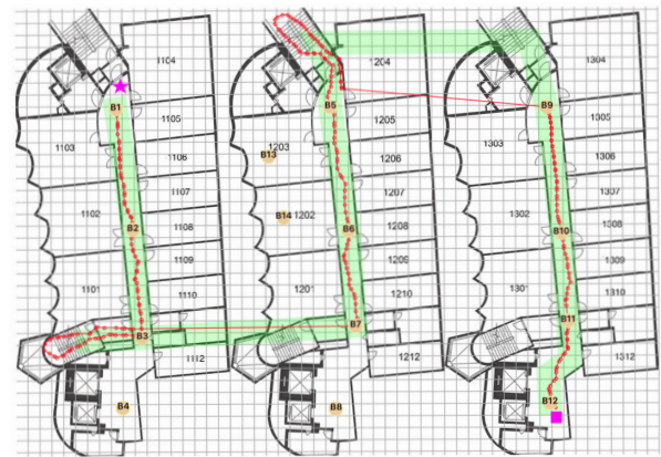
(a) Track 1: Floor detection with RSS-based profile.
