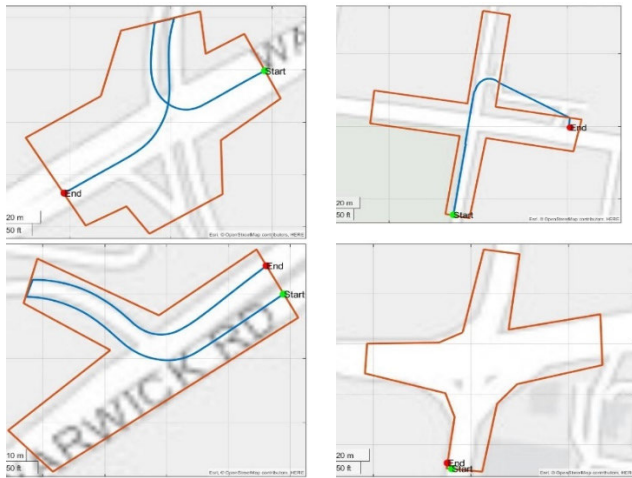
FIGURE 8. Some abnormal trajectories of intersection vehicle movements.
