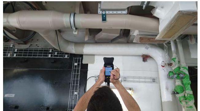
FIGURE 11. Testing of tag reading angles.
