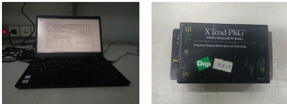
(e) Ground station (f) Telemetry hardware
