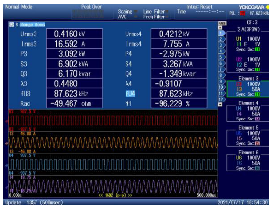
FIGURE 18. Test result of three-coil LCT with movable intermediate coil at the maximum offset.
