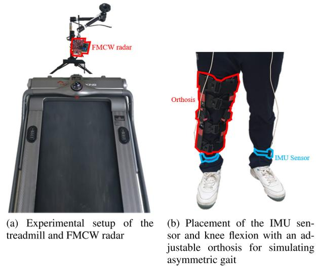
**FIGURE 6. Experimental setup of the treadmill and sensor configuration.**
