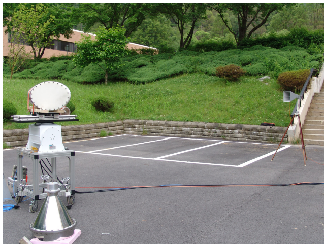
FIGURE 5. Cold test of a vlasov antenna.
