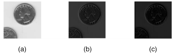
FIGURE 13. (a) Original image, (b) Image obtained from RTL simulation, (c) Image obtained from MATLAB.
