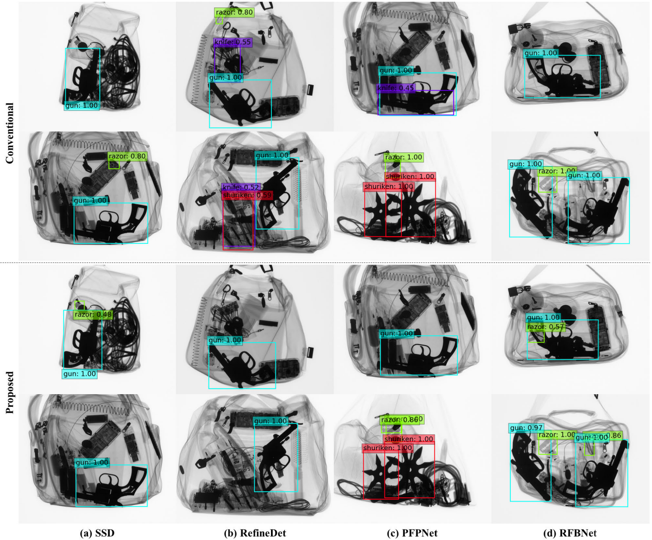
FIGURE 9. Examples of the real-world test results. Each colored box represents the detection result with the confidence score higher than 0.4.
