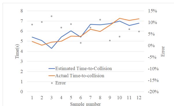
FIGURE 21. Line chart of estimated and actual times-to-collision.
