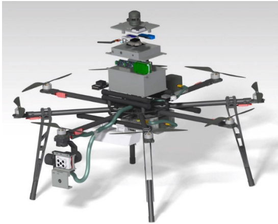
FIGURE 10. Details of UAV's mechanical system.
