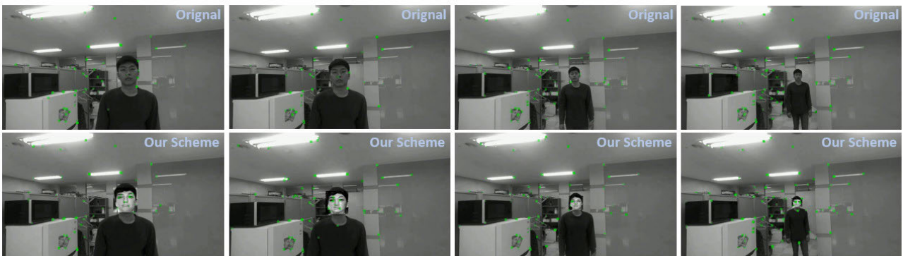
FIGURE 7. Feature points extracted by ORB-SLAM2 from the same videos in Fig. 6.
