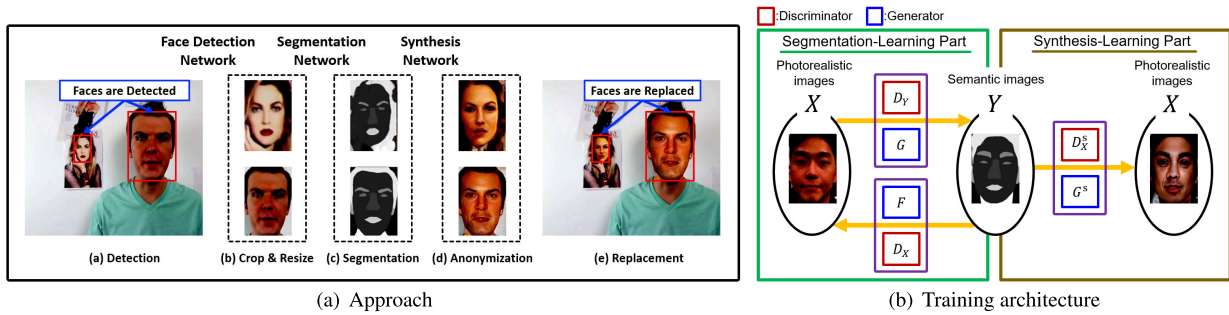
FIGURE 1. The proposed approach for anonymizing faces in a video frame and training architecture for segmentation and synthesis networks.
