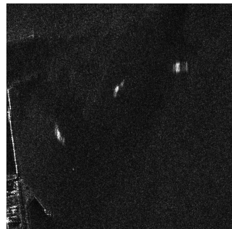
FIGURE 8. The deception jamming result of moving false targets with a large azimuth velocity.
