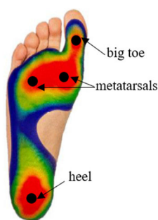
FIGURE 1. Typical plantar and shear forces distribution in the foot, with the areas with higher (red) and lower (blue) forces. Identification of the sensor-cells position (black dots).
