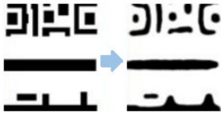
FIGURE 12. Edge distortion caused by limitations in the mask generation process in transition from the GDSII layout (left) to the silicon wafer (right) [54].
