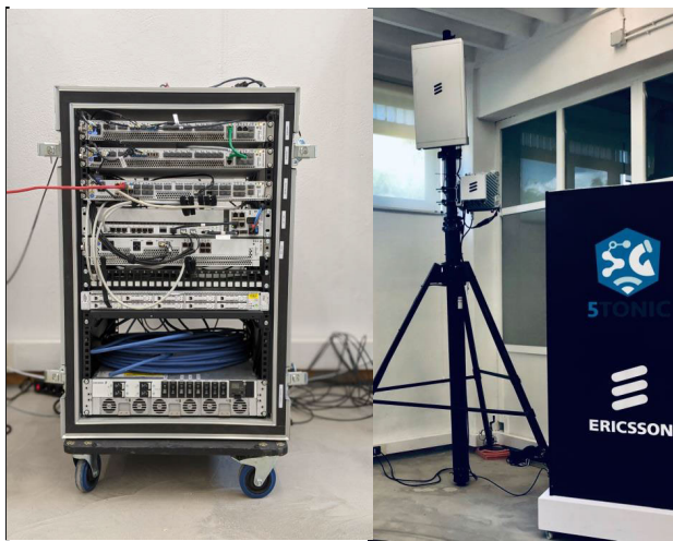
FIGURE 5. 5G NSA radio in the 5TONIC lab.
