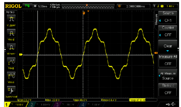
FIGURE 15. Back-EMF measured for a speed N \approx 480 rpm.
