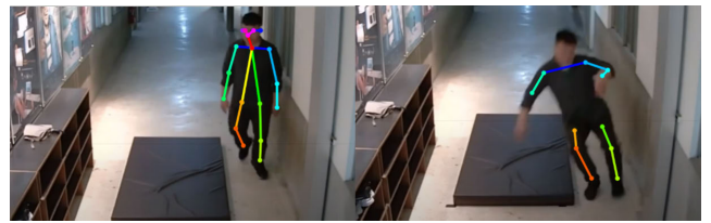
FIGURE 4. The human body in the image produces blurred areas when moving fast, resulting in the loss of some joint points.
