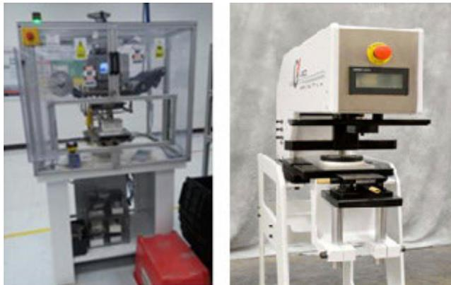
**FIGURE 8. Hot stamping machine and pad printing machine.**
