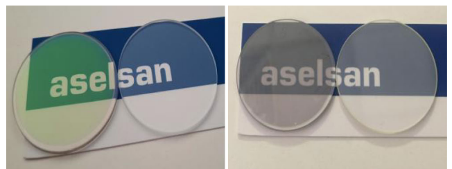
FIGURE 3. ITO coated B270 (left) and 4nm silver coated M-ZnS (right) with uncoated substrates.
