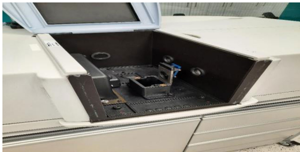
FIGURE 5. PerkinElmer lambda 950 UV/VIS spectrometer setup.
