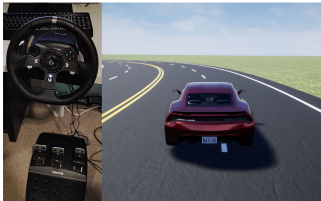
FIGURE 7. Driving controller and environment rendering in unreal engine for human demonstration.
