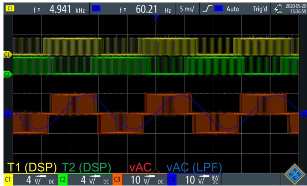
FIGURE 30. Waveforms of low voltage test of SMs connected in H bridge topology.
