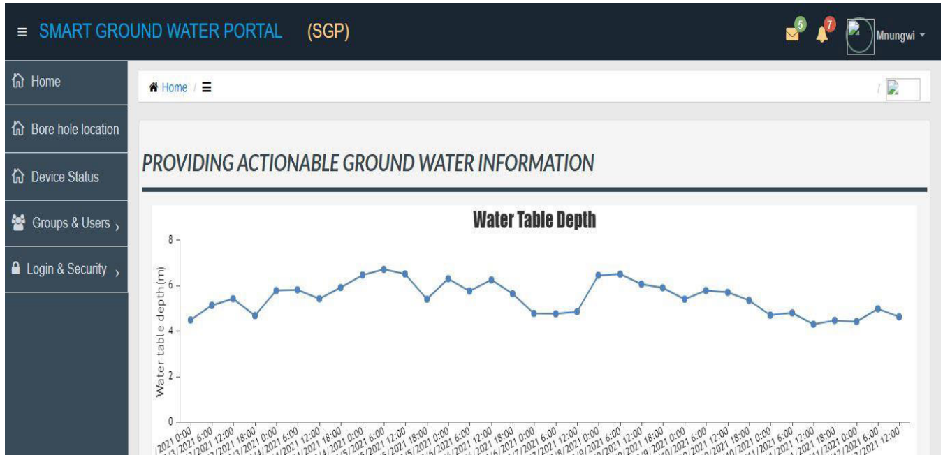
FIGURE 11. Web dashboard for LWNGM showing a plot of two weeks data from Bandamaji station at 6-hour intervals.
