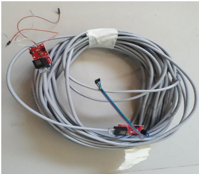
FIGURE 5. The I2C differential interfacing connectors attached to each end of the Cat 6 UTP sensor connection cable (25m).
