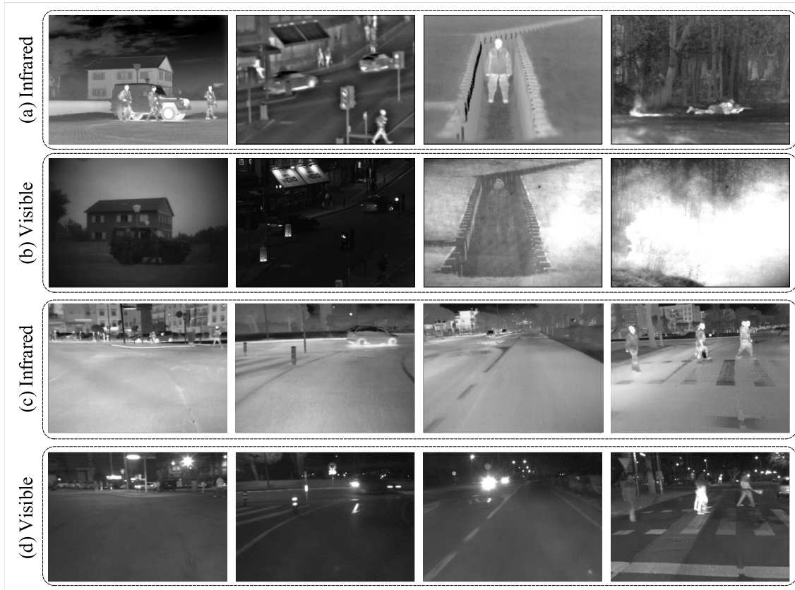
FIGURE 5. The examples of infrared and visible images in the TNO and CVC-14 datasets. All images have been registered. (a) and (b) is the infrared and visible images examples of TNO dataset; (c) and (d) is the infrared and visible images examples of CVC-14 dataset.
