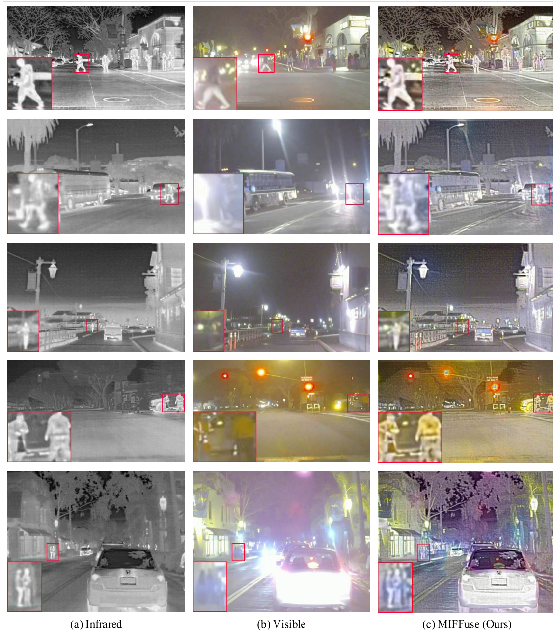
FIGURE 13. Fused results for infrared and visible (RGB) images. (a) Infrared image; (b) Visible image; (c) Our MIFFuse.
