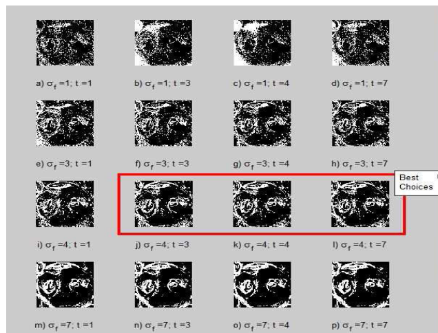
FIGURE 6. Impact of DGau pre-filtering and texture quantization on the muzzle of a Ghungroo pig (Fig. 5).
