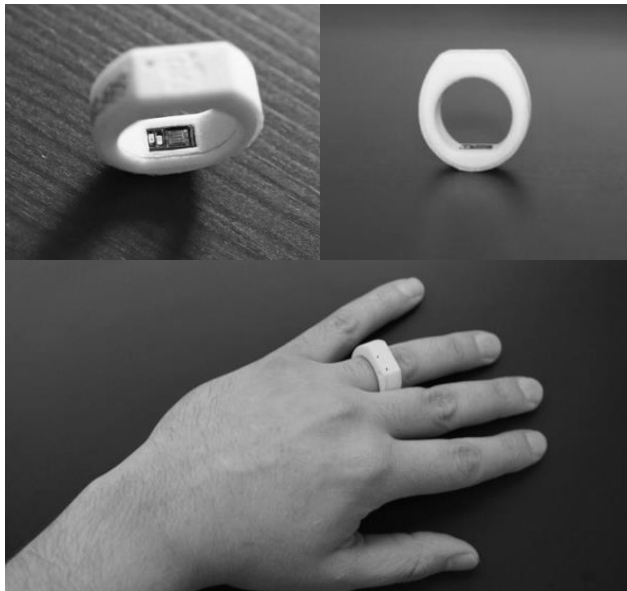
FIGURE 10. Photograph of the ring device embedding the presented monolithic sensor and its optimized optical module.
