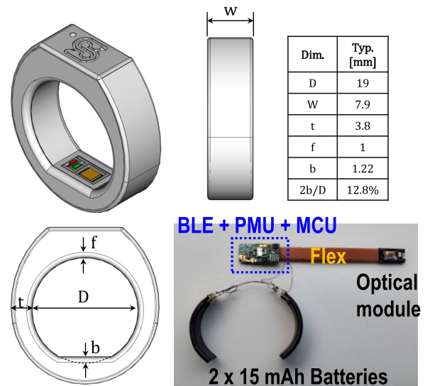
FIGURE 7. Isometric and orthogonal views of the ring, including teardown of the electronic system.
